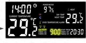
NIGHT FROM set the time when you would like night temperatures to run from. Set the hours then press SET and repeat to adjust minutes.
