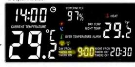
TIMER1 OFF set the time when you would like No.1 timer to switch off. Set the hours then press SET and repeat to adjust minutes.
