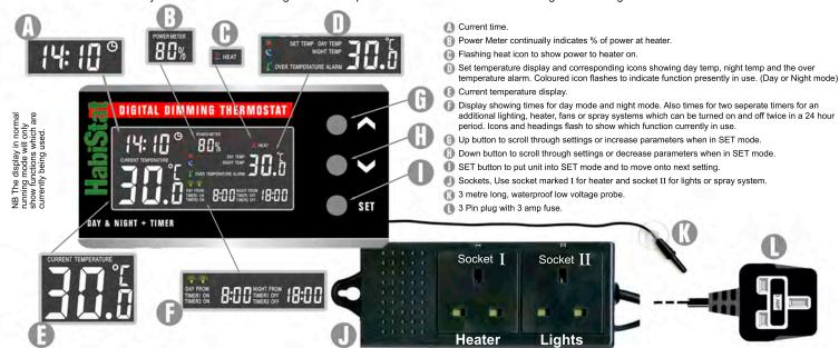
**SETTINGS**. Press the **SET** button and hold for 3 seconds. This puts the unit into SET mode. Use the **Λ V** buttons to change parameters (hold button down for rapid change) and then press **SET** to save and move onto the next setting. The order is shown below. Elements highlighted indicates flashing display.
